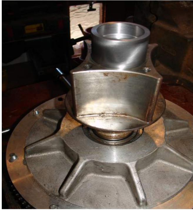
The stub shaft bolted in position.
