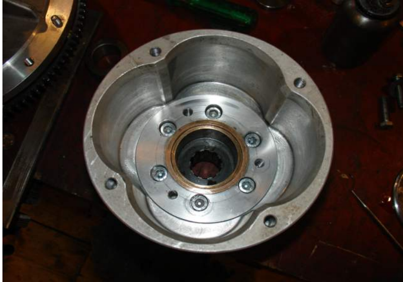
Inside the Centa outer rotor showing the bearing carrier in situ
