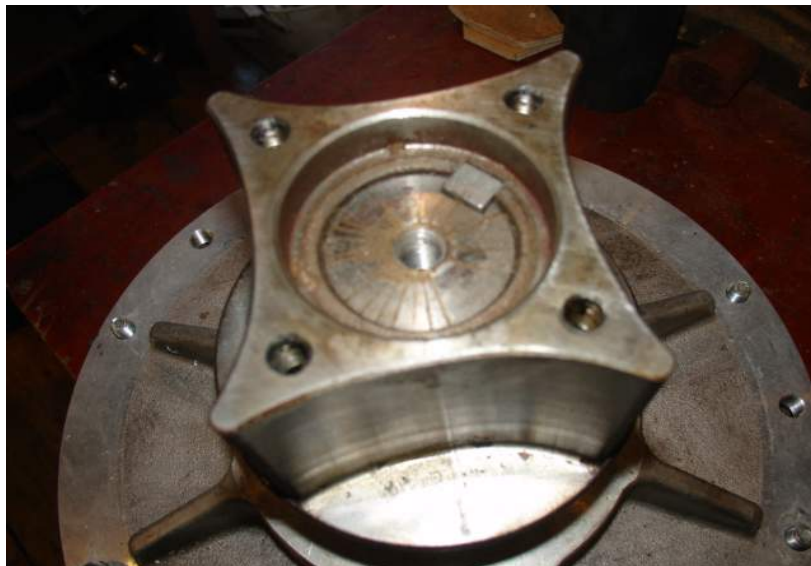
The inner Centa rotor showing the recess for the stub shaft and the front plate removed
