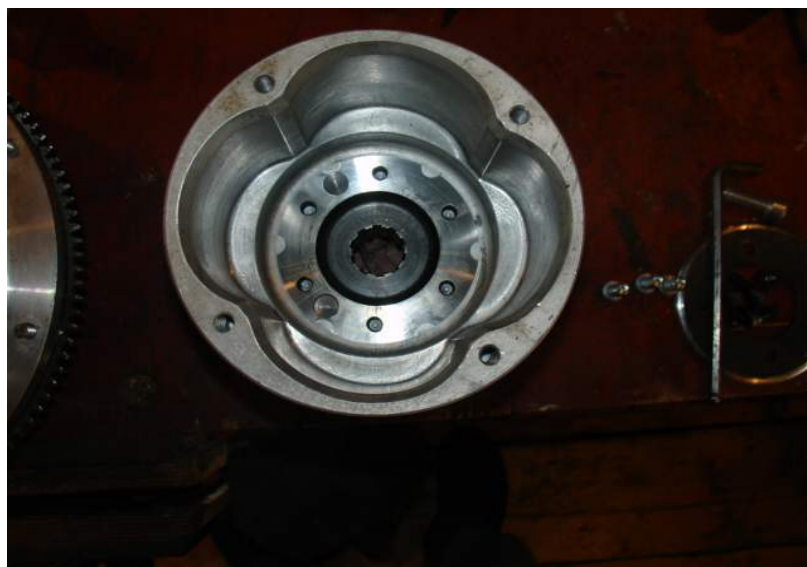
Inside the Centa outer rotor showing the recess for the bearing carrier
